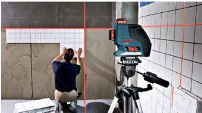
Horizontal Laser Plane
