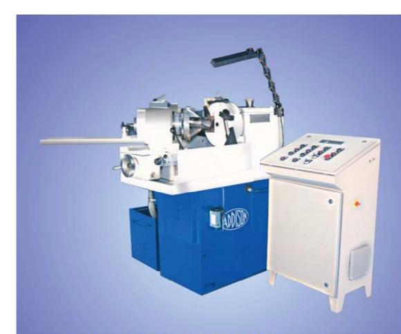
Addison Automatic Drill Point Grinder Model ADG 80 & ADG 100 are a versatile compact & sturdy machine and designed for sharpening the Point of the Twist Drills in a wide range of Two, Three & Four flutes accurately and quickly. This machine can accommodate drills From Diameter 10mm to 80mm(for ADG 80) and 10mm -100mm (for ADG 100) with overall length up to 1000 mm.
